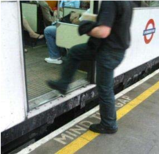
The picture above is an example of a rail stop that lacks a ramp. This makes entering & exiting very difficult for seniors and impossible for wheelchair-bound individuals.
